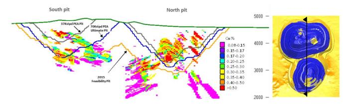
Long-section of PEA Pit for 37Kstpd Initial Mine Plan and Expanded 70Kstpd Ultimate Pit.
